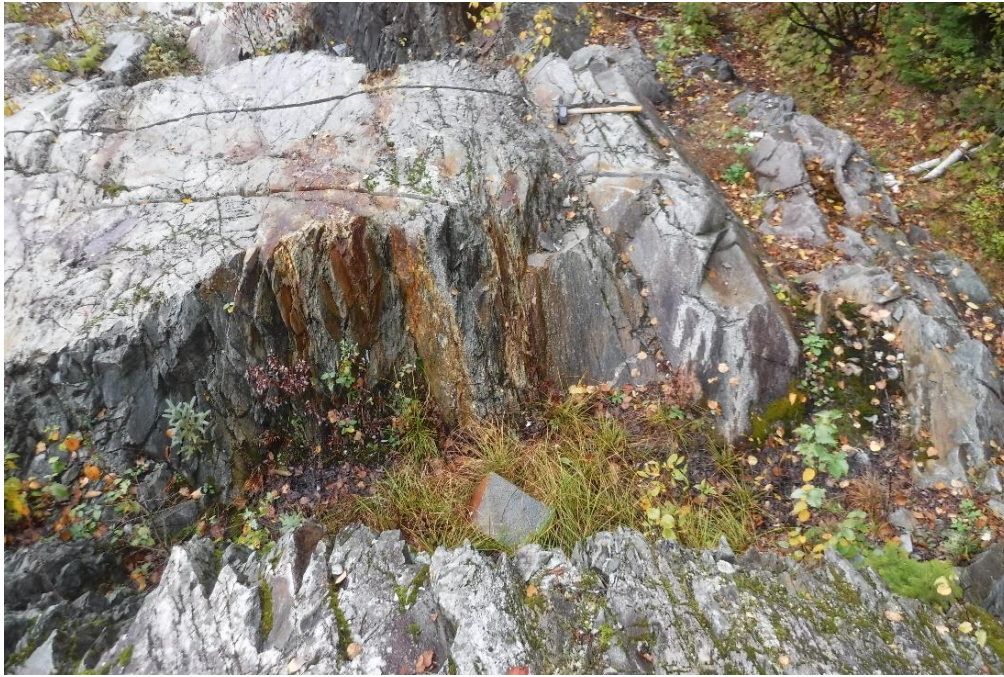
Figure 21: Patchy, pinch-and-swell, and iron-stained zone of disseminated pyrite and pyrite stringers hosted in west-trending steeply dipping shear zone crosscutting a feldspar porphyry intrusion within Golden Share stripped area GSH-11-A
