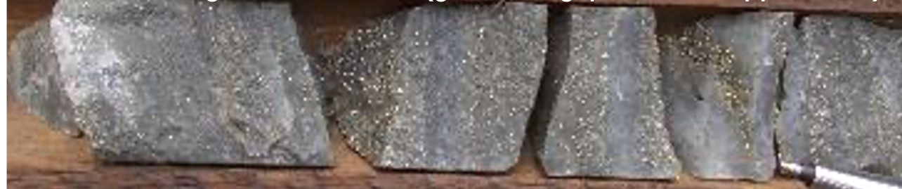
McKinnon main gold zone host rock (gold bearing quartz-sericite-pyrite schist)
